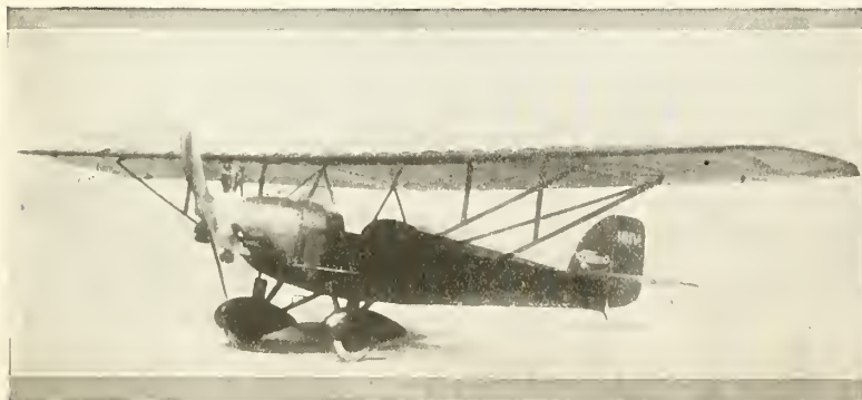
The new convertible Corben Junior Ace two-place side-by-side open type monoplane
